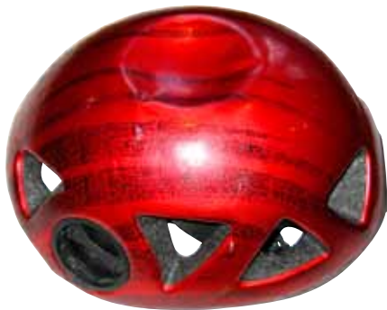
Foam helmet after impact testing
