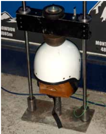
Testing an old Joe Brown hardshell helmet
