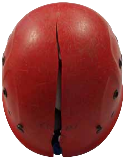
Old plastic shell after impact testing
