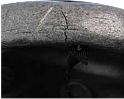
Cracked foam helmet
